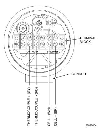
Figure 5-2. Oxygen Probe Terminal Block
